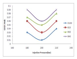
Figure 5: Influence of injection pressure on CO emissions
