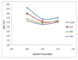
Figure 4: Influence of injection pressure on exhaust gas temperature
