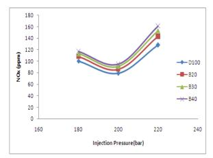
Figure 7: Influence of injection pressure on NOx emissions
