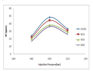
Figure 6: Influence of injection pressure on HC emissions
