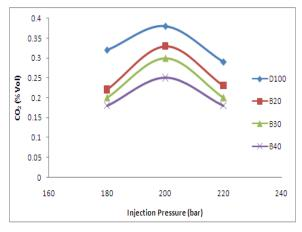
Figure 8: Influence of injection pressure on CO<sub>2</sub> emissions
