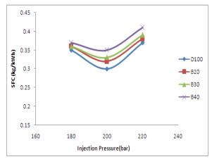
Figure 2: Influence of injection pressure on specific fuel consumption
