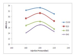
Figure 3: Influence of injection pressure on Brake thermal efficiency
